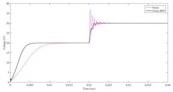
Fig. 9 Servo Responses of Luo Converter with Controllers.
