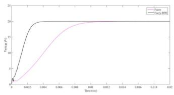
Fig. 6 Step Responses of Luo Converter with Fuzzy and BFOA-fuzzy Controllers
