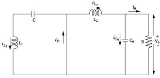
Fig. 3 Equivalent Circuit During Switch-OFF (Mode 2)
