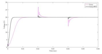
Fig. 7 Responses of Luo Converter for  $\pm$  25% Line disturbances
