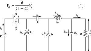
Fig. 1 Circuit Diagram of Positive Output Elementary Luo Converter
