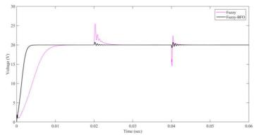
Fig.8 Output Responses under  $\pm$  20% Load Disturbances
