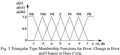
The derivation of the fuzzy control rules is heuristic in nature and is shown in Table 1. The inference mechanism seeks to determine which rules fire to find out which rules are relevant to the current situation. The inference mechanism combines the recommendations of all the rules to come up with a single conclusion.
