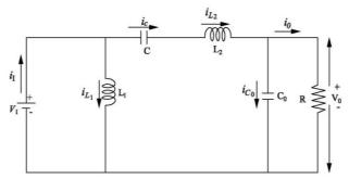
Fig. 2 Equivalent Circuit During Switch-ON (Mode 1)
